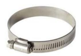
Constructed with all 300 grade stainless steel, the lining of these clamps protects the hose surface and prevents silicone from shearing through band notches. The clamps are salt water resistant, making them an ideal solution for marine applications.
