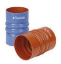
This charge air connector for the hot side features 4-ply silicone coated meta-aramid fabric with stainless steel pressure retention rings.
