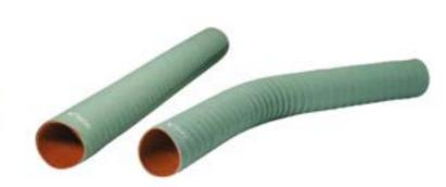
This coolant hose is reinforced with two plies of polyester reinforcement, with helical wire that allows for some forced curvature. This design makes it an ideal solution for heavy duty pressure connections in hostile engine environments.
